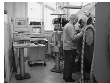
Fig. 2 Computer-controlled vacuum plasma spray equipment with in-flight particle diagnostics and four-fold powder feeder
